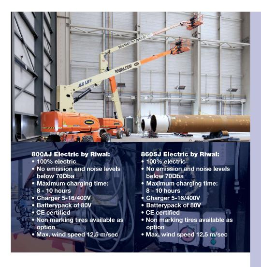
Riwal is offering much more than only standard machines. We customise machines based on customer demand. The conversion of the JLG 800AJ and the JLG 860SJ are great examples. Developed in close cooperation with customers with specific needs, these machines are a sustainable alternative to diesel powered machines. Zero emissions and low noise levels are beneficial to the environment as well as the machine operators.
